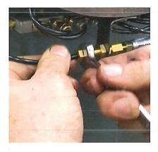
5. Use a 10mm wrench to tighten the compressing bushing onto the rubber hose.
