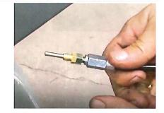
7. Install the rubber hose into the 4-way junction block and use a 3/8" wrench to tighten into the junction block.
