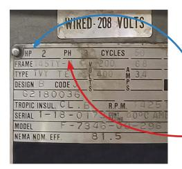
In order to determine your Bridgeport Machine type, we need to start with the motor. Use the diagram below to help you locate the HP of your Bridgeport Machine Motor.
