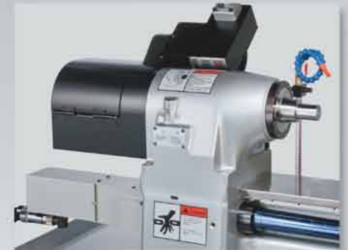
Air operated collet closure (with foot switch) is provided as a standard accessory for quick and easy release of a workpiece. A pull-down style chip guard protects the operator from flying chips. Full length splash guard is mounted at the back to contain coolant splashing and flying chips.
