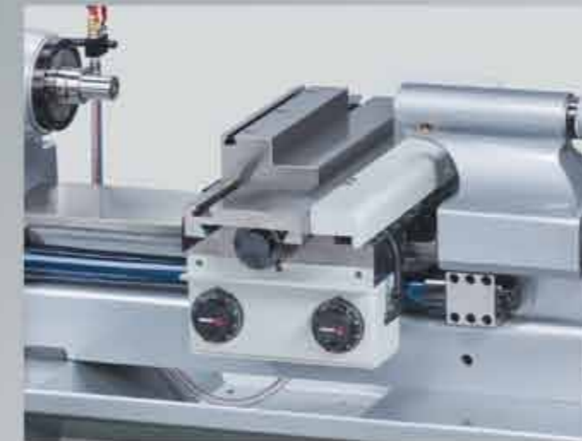
Gang-type machining showing additional tool plate (standard) mounted on top of cross slide, equipped with various tool holders and tools (optional).
